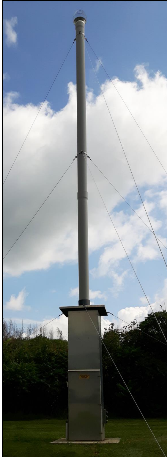
Figure 5.1. The Brock University Rothamsted Trap. Insects are captured at the top of the trap via suction and brought down into a collection bottle, housed within the rectangular base.
