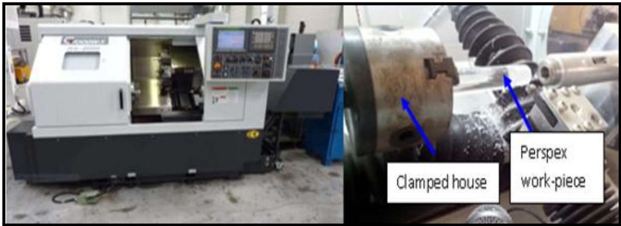
Fig. 1: Experimental setup for Perspex turning operation
