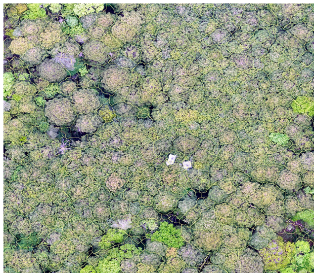
Figure 7. Results of the watershed segmentation method for delineating the individual canopy area. Although slight differences in segments can be seen, overall, it can perform extraction rather well even in the highly dense forested areas.
