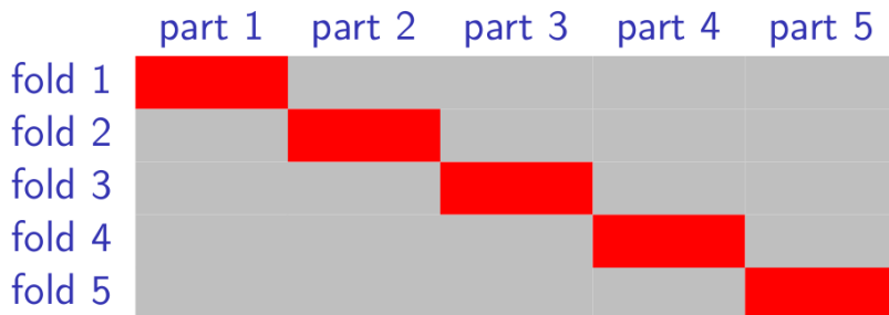
Figure 3: Illustration of 5-fold cross validation, the grey squares are the training set and the red square represent the evaluation set.
