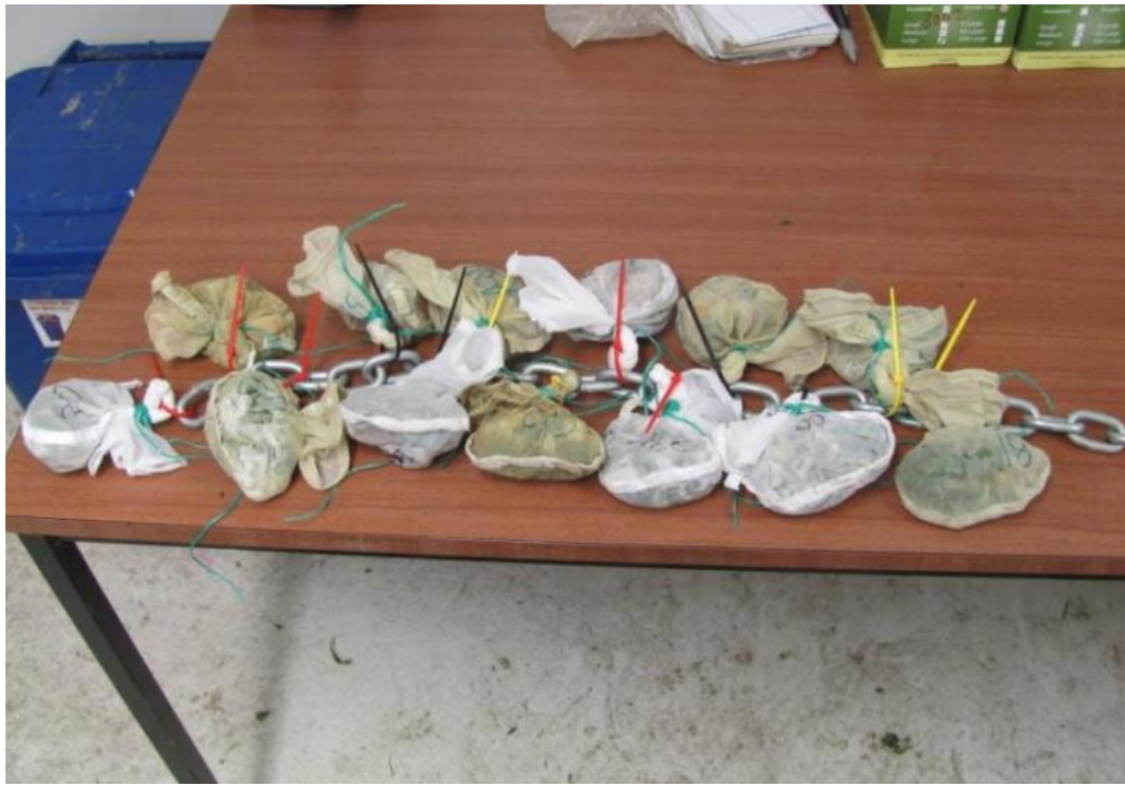
Plate 5.1 Cut herbage in dacron bags attached to alternate galvanised chain links by cable ties.
