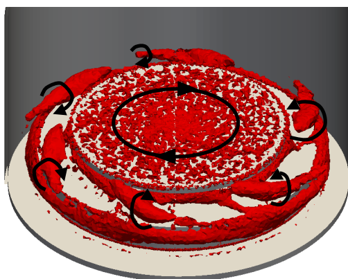
Fig. 1 Snapshot of large-scale vortex structures observed in a modeled single spin cleaner. The vortical regions are identified with the second invariant of velocity gradient tensor over 200 for LES. The disk rotates in a clockwise direction in this figure (Kouchi, et al., 2015).
