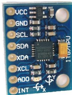
(g) Sensor MPU6050 [Arduino, 2018d]
