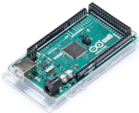
(a) Arduino MEGA2560 [Arduino, 2018a]
