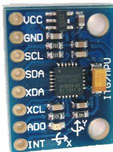
(c) Sensor MPU6050 [Arduino, 2018d]
