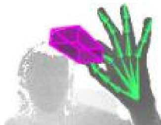
Figure 3.3: Example of mesh based hand model holding an object. Extracted from [SMZ + 16].
