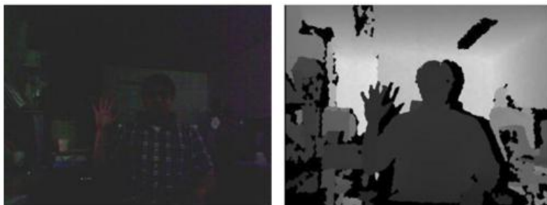
Figure 3.6: Comparison between colour and depth images in a low illuminated scenario. Adapted from [PYK + 12].
