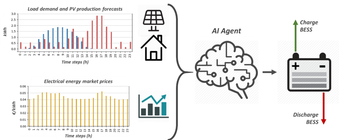
Figure 1 - Flow diagram of the implementation of AI to the predictive storage control problem. The AI agent takes as inputs a set of consecutive load demand and PV production hourly forecasts along with the evolution of electrical energy market prices for the corresponding hours, outputting an action, for the current time step, that translates into a charging or discharging energy that will be required from the BESS.
