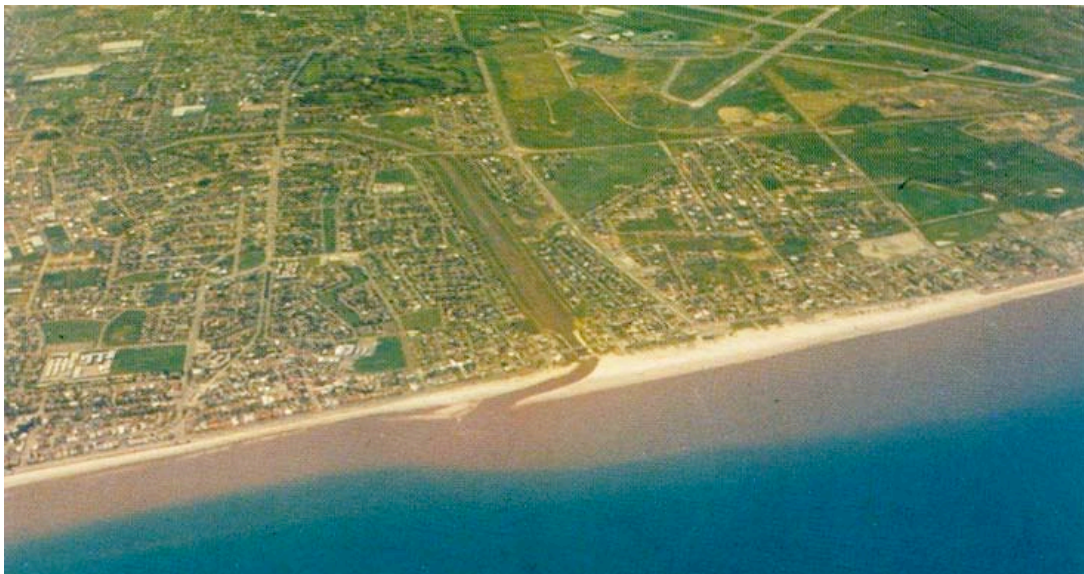
Figure 6.1: Photograph of Torrens River outflow into Gulf St. Vincent during a flood in October 1974. Sediment plume travels northwards (towards head of gulf) due to longshore drift. Photograph from (Lewis 1975).
