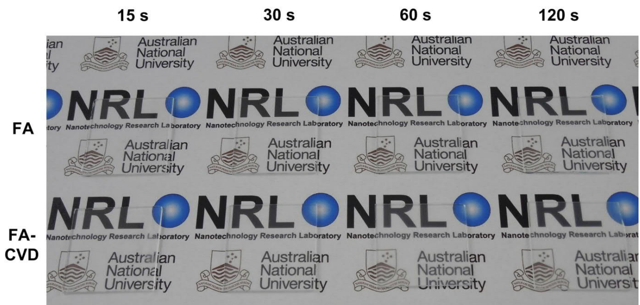
Figure S8.5. Optical images of coatings. Photographic images of (1 st row) FA and (2 nd row) FA-CVD developed nanoparticulate coatings. Deposition was optimized across (1 st column) 15s to (4 th column) 120s while preserving > 80% transmittance. NRL logo, copyright A. Tricoli. ANU logo, copyright the Australian National University.
