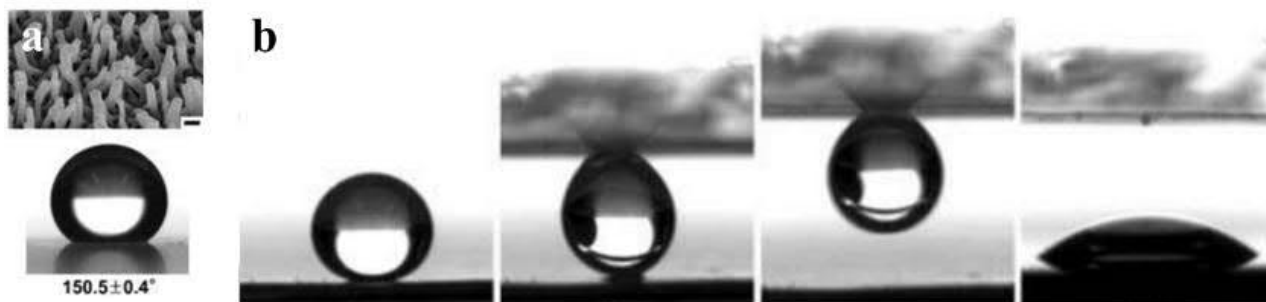
Figure 2.43. Superhydrophobic petal-effect properties. a) Nanotubular morphology b) Nanotubular surface demonstrating mechanical hand-like properties. [138]
