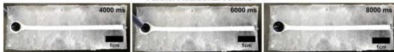
Figure S7.11. Response of the PVC side of the Janus bilayer to water. The wetting characterization of the opposing superhydrophobic PVC side of a 2 mm-wide strip of Janus bilayer on superhydrophobic nanofibrous substrates reveals no Mimosa Origami self-assembly.
