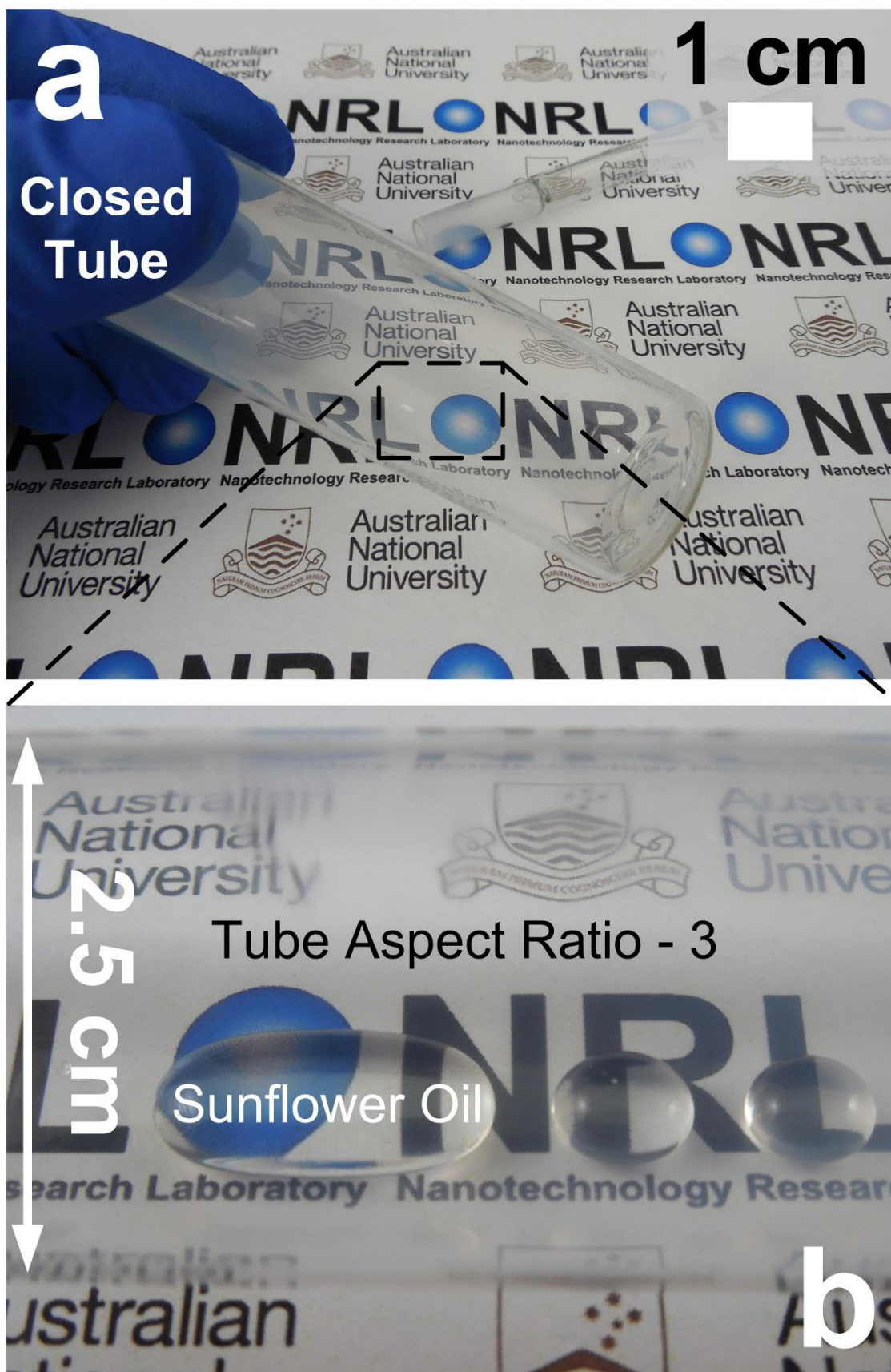
Figure S8.9. Exemplified coatings. a) Inner walls of a closed cylindrical tube, with a b) moderate aspect ratio ( L/D ) of 3, showcasing the omni-directional suitability of these super-oleophobic (-amphiphobic) coatings.
