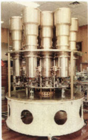
Fig. 2.2: Photo of the Parkes Multibeam instrument (left) and the configuration pattern of the 13 receivers in the instrument (right). The angle between the receivers and the radius on the sky of the inner and outer receiver rings is shown on the configuration diagram. Both images are taken from the Multibeam survey web site, http://www.atnf.csiro.au/research/multibeam/ .
