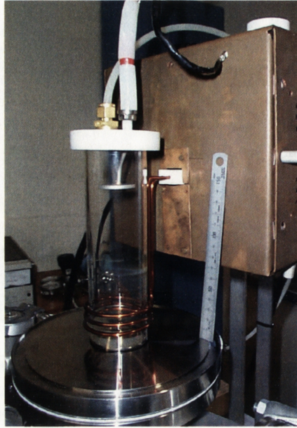
Figure 4.5: A close-up view of the discharge tube. The electrode that sets the plasma potential can clearly be seen at the top of the tube. The antenna is at the bottom of the tube near the extraction orifice. The square box houses the matching network.
