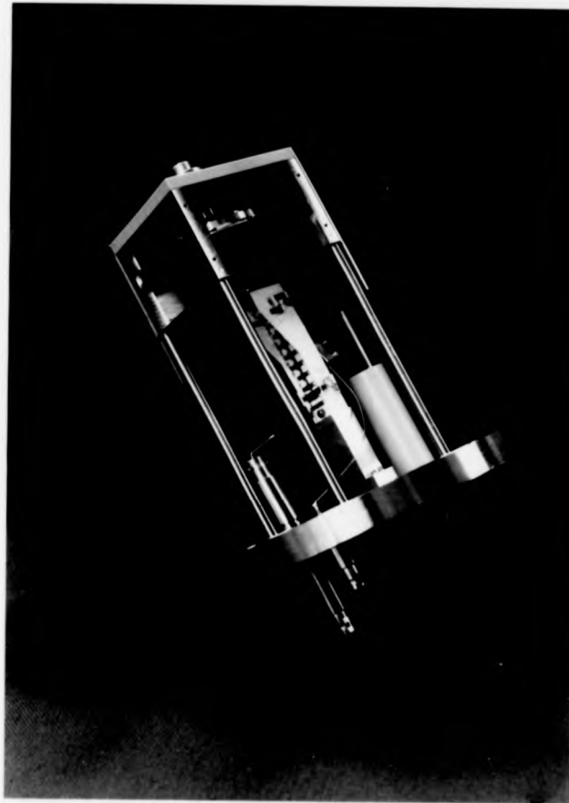
Figure 3.5.1.(1a) Photograph of the off-axis post-acceleration detector.
