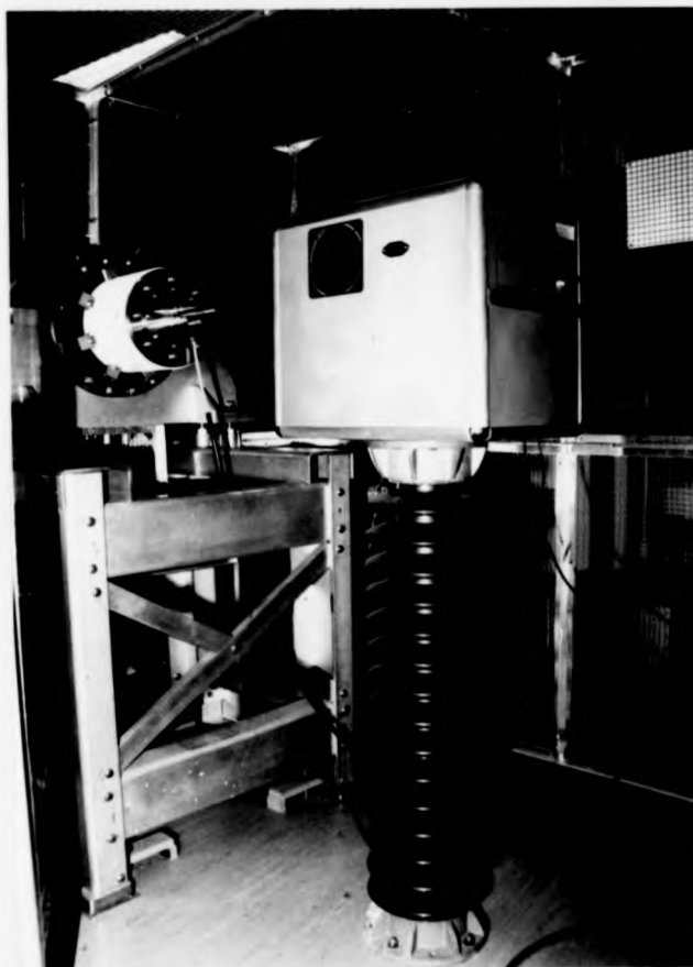
Figure 3.1.3.(1) Photograph of the Faraday cage at the end of the ER-TOF instrument
