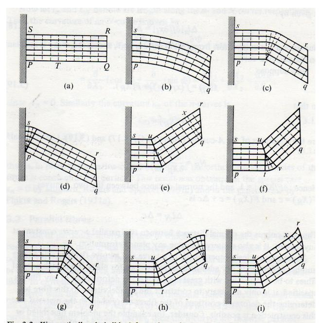
Fig. 3.2. Kinematically admissible deformations of a rectangular block. Solid lines denote *a*-curves, broken lines denote *n*-curves.
