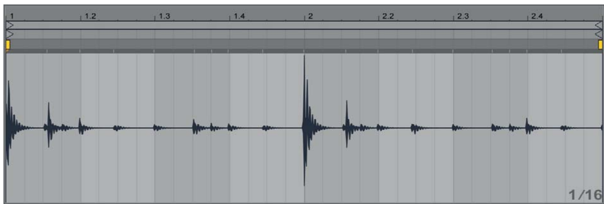
Abb. 3: Clock-Signal am Audio-Ausgang des Rhythm King (Screenshot in Ableton Live). Quelle: Screenshot in Ableton Live , Malte Pelleter
