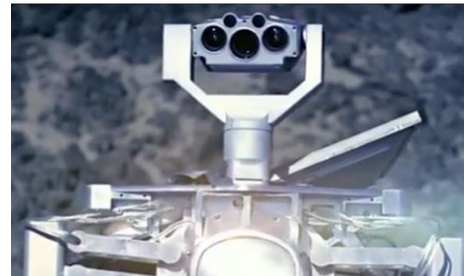
Figure 1: Compact Lidar Spectrometer Will Look Similar to Camera Mounted on a Rover (PT Scientists). The CLS can be mounted and coaligned with the camera system.
