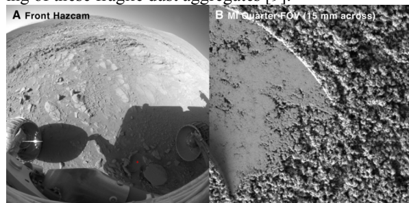
Figure 3. Mössbauer contact plate impression into dust mantle at Gusev crater. (A) front hazcam with red dot showing MI image location; (B) quarter-frame excerpt of MI image, ~15 mm across. Large, well-developed dust aggregates blanket the regolith. MI view shows where the Mössbauer contact ring touched the ground with ~1 N of force, completely and easily crushing the aggregates into ultrafine, unresolved particles that allow a high-fidelity casting of the smooth metal surface of the contact plate. (After Fig. 20 of [9])
