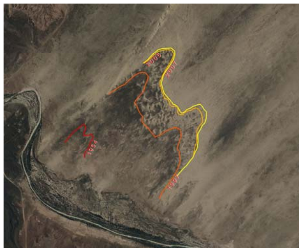
Figure 2. Migration of Grand Falls dune field based on 1954 (red) aerial photo, 1997 (orange) and 2005 (gold) DOQQs and 2007 (yellow) NAPP. Between 1954 and 2007, the dune field moved ~1.6 km. Figure back-ground is 2007 NAPP.
