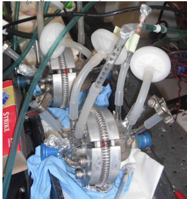
Figure 2: Fuel cell experiments to simulate geochemical seafloor interfaces on Europa or Enceladus.
