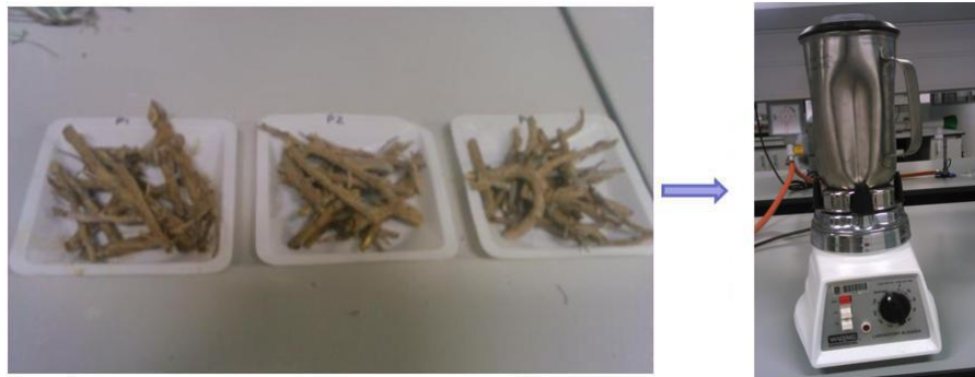
Figure 3.2: Guayule latex extraction: Latex extractions were done in triplicate for all the lines using extraction buffer (KOH pH 11) in a Waring blender
