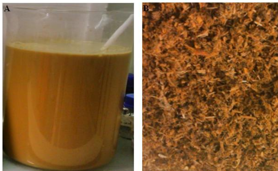
Figure 3.4: The latex homogenate from stem extractions: a The latex homogenate after filtration. b The bagasse with good hemicelluloses content was obtained as a by-product.
