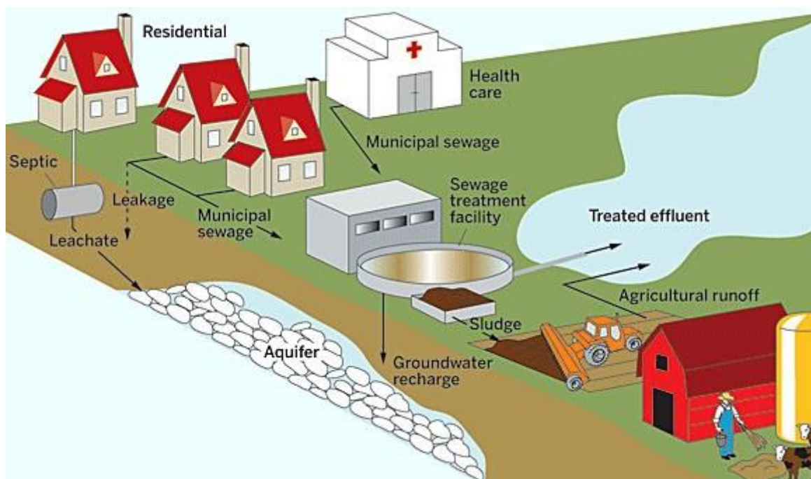
Figure 1. 4: Schematic of EDC and PPCP leakage into drinking water ( www.eusem.com ) (J. Lintelmann, A. Katayama, N. Kurihara, L. Shore, A. Wenzel, Endocrine disruptors in the environment (IUPAC technical report), Pure Appl. Chem. 75 (2003) 631–681.).
