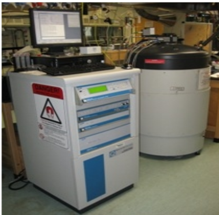
Figure 3.5: A commercial Quantum Design Physical Property Measurement system (QD PPMS), University of Johannesburg, Department of Physics.
