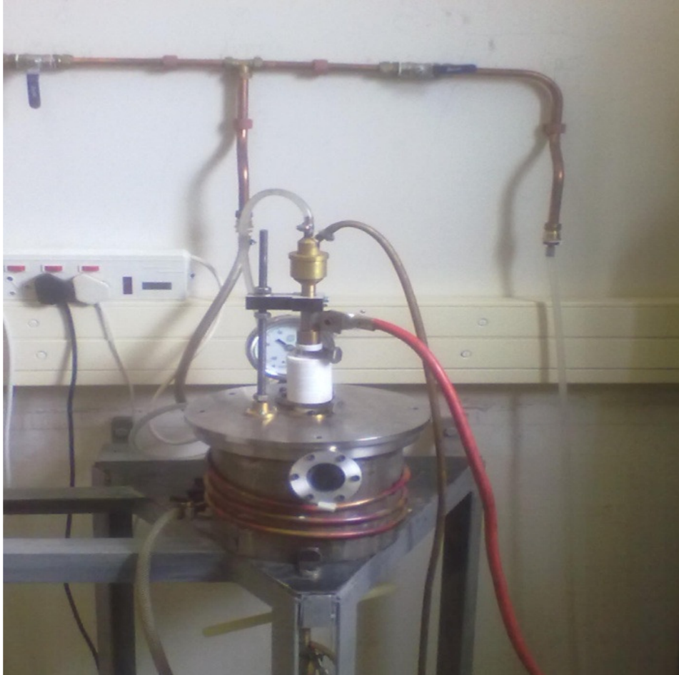
Figure 3.1: Arc-melting furnace chamber at the University of the Western Cape (Physics Department).
