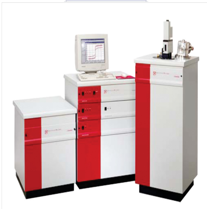
Figure 3.6: A Superconducting Quantum Interference Device (SQUID) magnetometer in a Quantum Design Magnetic Property Measurement System (QD MPMS-5).
