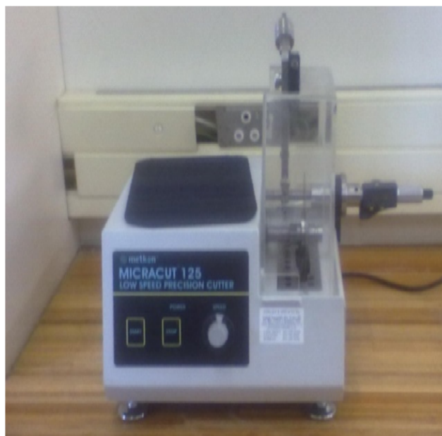
Figure 3.3: Micracut 125 low speed cutter at the University of the Western Cape (Physics Department).
