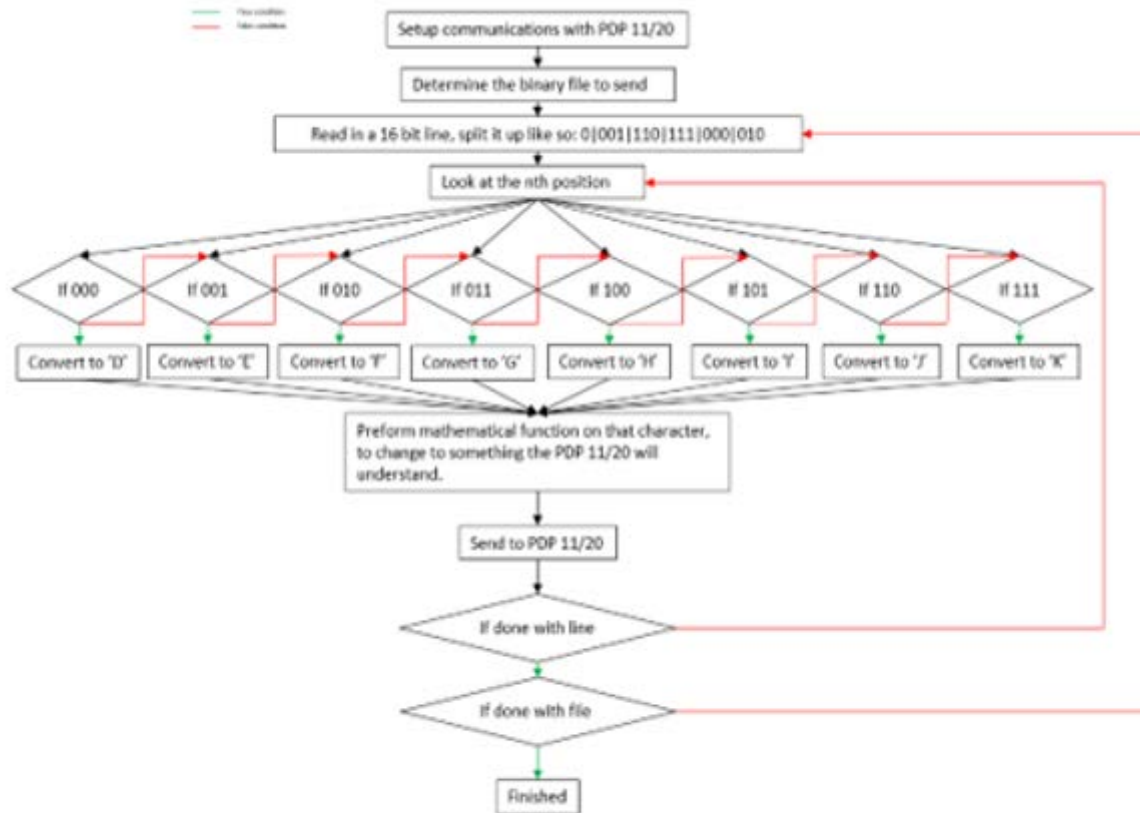
Figure 20: The above flowchart depicts how our serial console sends the information from our BASIC binary file from our laptop to the PDP 11/20
