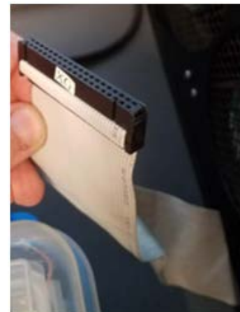
Figure 14: The 40-pin berg cable classically would allow communication between the PDP 11/20 and a peripheral device.
