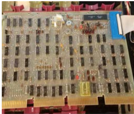
Figure 13: The DL11 serial interface card which is stored in the chassis of the PDP 11/20, and handles communication between the PDP, and an external peripheral device.
