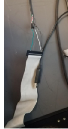
Figure 15: The serial adapter is attached to the ground, TX, and RX lines on the berg cable, and is used to allow communication between our laptop, and the PDP 11/20.
