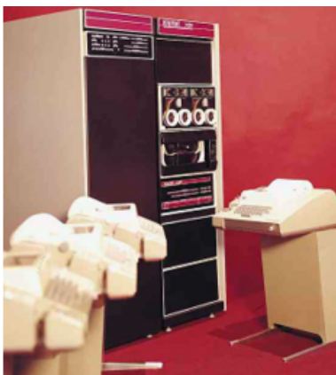
Figure 1: An image of the original PDP 11/20 that was sold in 1970. The main interface beign a series of LED's and switched shown on the middle right. Above that are the paper tape I/O devices.
