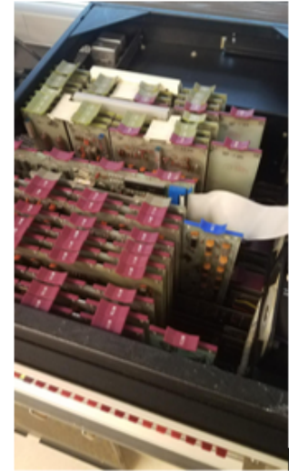
Figure 6: The internal structure of the PDP 11/20. Each interface card is attached to the UNIBUS below. Interestingly, the UNIBUS runs along the top part of the chassis, and the cards hang down from it. To examine the inside of PDP 11/20, it must first be flipped upside down.
