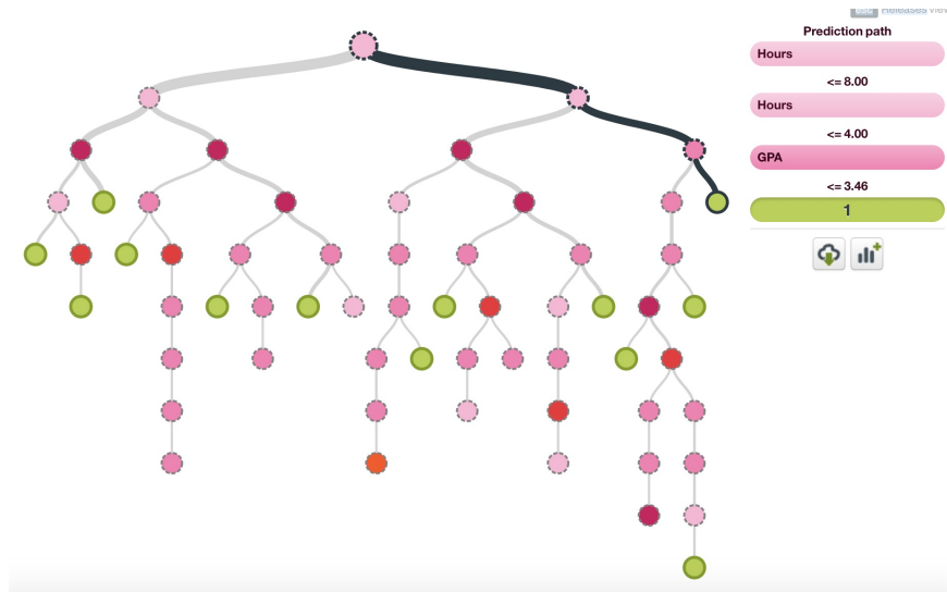
Figure 1: Screenshot of the tree diagram for the generated dataset that was generated through BigML. The bold path that leads to a green dot is the path that the model took in order to predict a specific group of customers as a "1." The individual steps that were taken in that exact instance are shown in the far right upper corner.
