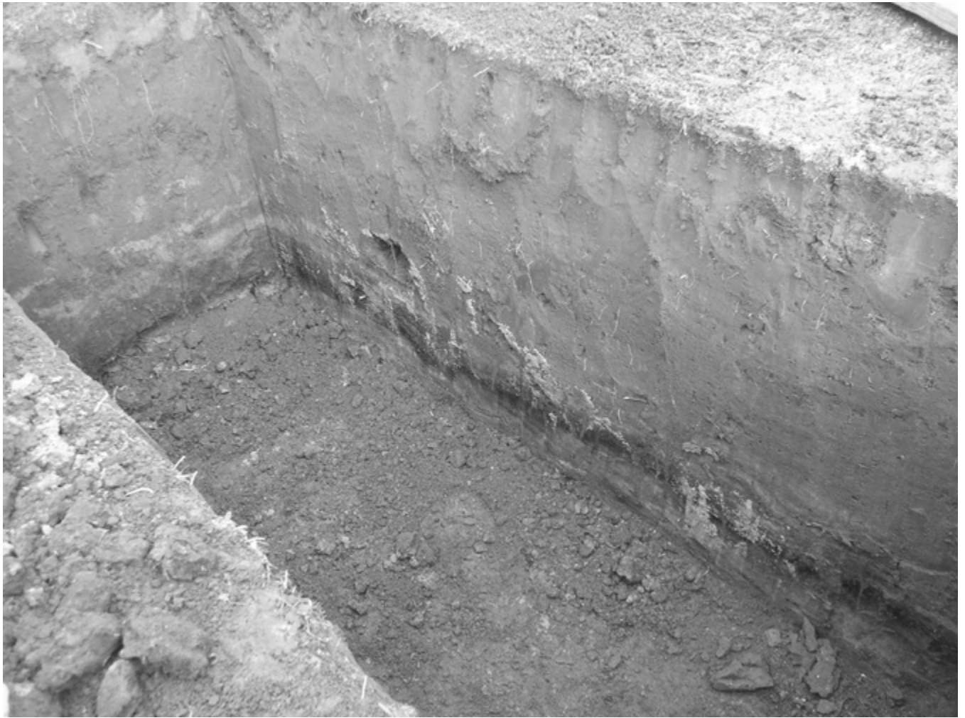
Figure 4. Section of Trench Showing Soil Horizons
