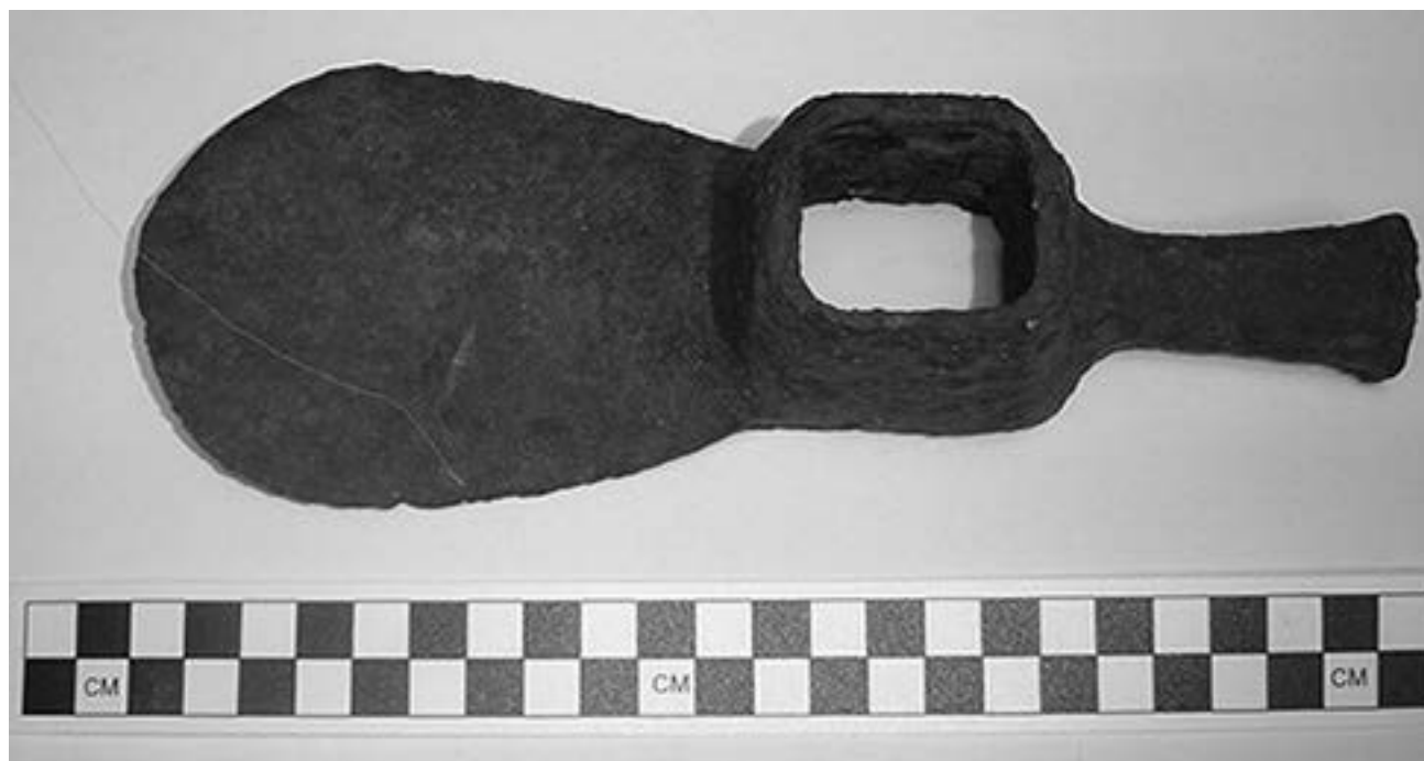
Figure 2. ca. 1800 iron adze blade used to build ships made by Joseph Holmes from 1801 to 1806 at his Bridgewater Shipyard. This adze is 8 3/4" (22.2cm) long by 3 1/8" (7.9 cm) wide, with a 2 1/4" (5.7 cm) hammer, 1" (2.5 cm) wide. Photo by David DeMello
