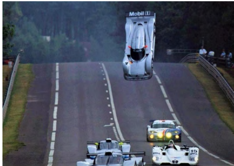
Figure 1: Mark's Webber accident at the Circuit de la Sarthes due to the car suffering of aerodynamic instabilities along the circuit's long high-speed straight sections, Le Mans 1999
