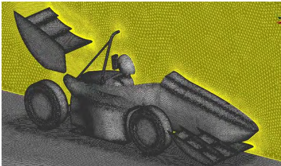
Figure 83: Surface mesh created for the final model
