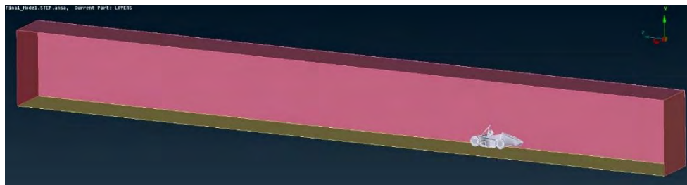
Figure 76: Fluid Domain of the CFD model for Sidepods & Undertray
