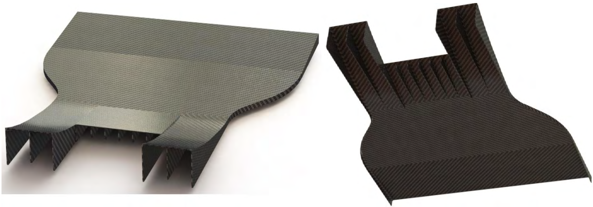
Figure 117: Separated diffusers CAD designs
