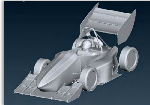
Figure 81: CAD model of the car with full aerodynamic package
