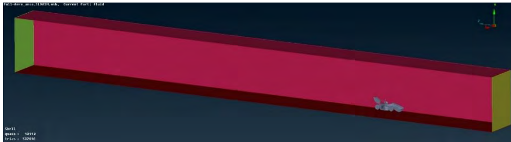
Figure 82: Fluid Domain of the final CFD model
