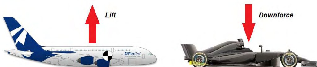
Figure 2: Race cars use inverted airplane wings to produce downforce instead of lift
