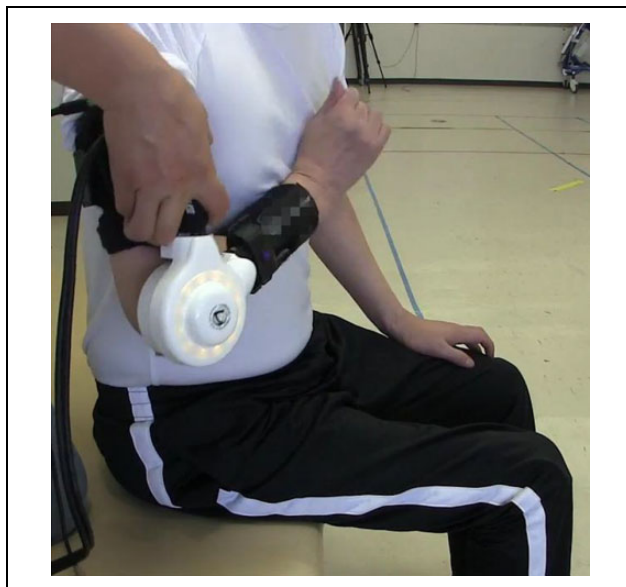
Figure 5. Elbow flexion exercises using the upper limb HAL-SJ in case 2. HAL-SJ: single-joint Hybrid Assistive Limb.
