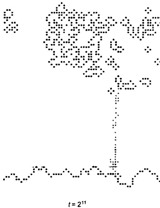
Figure 2. Morphology of the random solid system at t=2^{11} . Dark gray scale represents the random solid and the light gray scale represents the solution. Black dots are the externally accessible perimeter sites in contact with the solution. The solid line represents the lattice boundary at t=0 .
