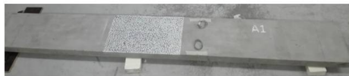
Slab A1: RC slab control specimen
