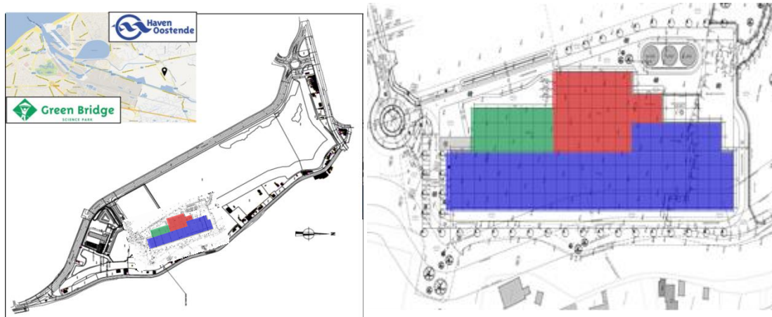
Fig. 2. Top - Location of the upcoming physical modelling research cluster near the port of the Ostend. Bottom - red upper right part: COB main hall, blue lower part: towing tank, green upper left part: shared office space.
