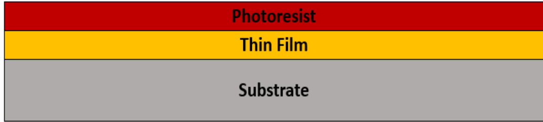
Figure 3-7: Step 2 Lithography Preparation
