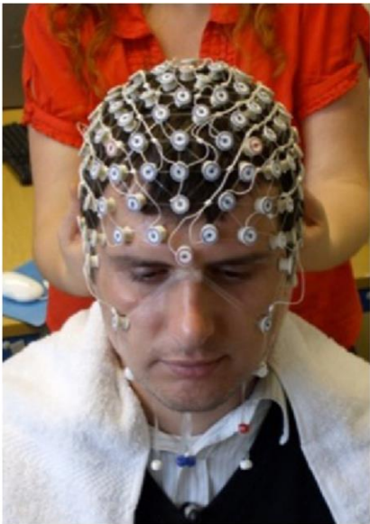
Figure 8. Example of the Electrical Geodesics Incorporated 128-channel electroencephalographic Geodesic Sensory Net participants wore throughout the experiment.
