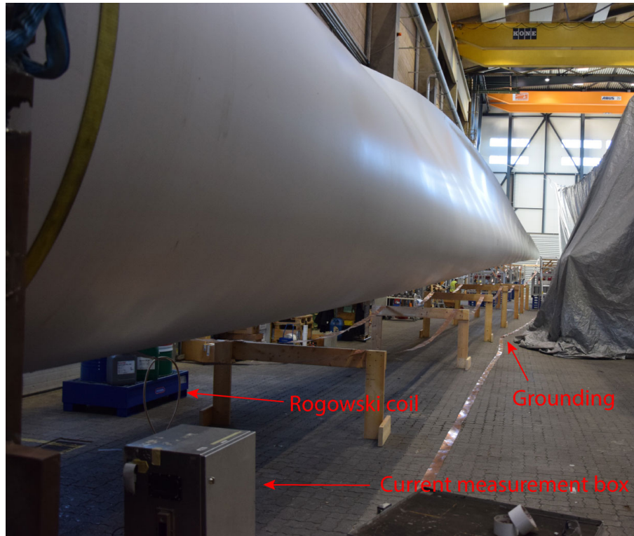
Figure D.3: Picture from the root end towards the tip of the blade. Current measurement is performed with Rogowski coils. The root of the blade is grounded.
