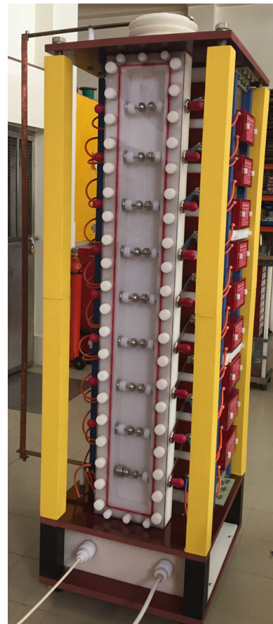
(b) Picture of D-bank. View shows encapsulated spark gaps and resistors. Terminals are short circuited.
