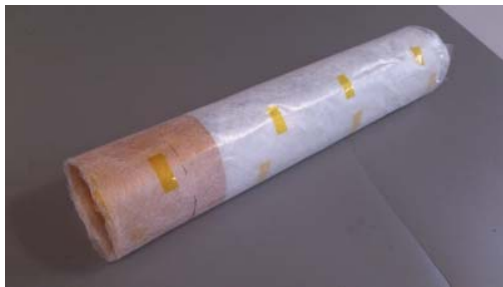
Figure 2. MLI added around the inner tube of the cryostat to prevent heat losses through radiation. It contains a part with regular aluminized Mylar, and a smaller part with Kapton film.
