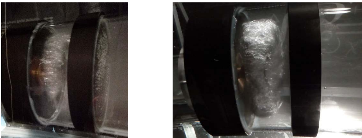
Fig. 12 Visualisation of the vortex ring between the catalyst dummy and the expansion. The flow is from left to right.
