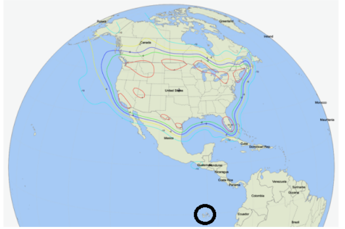
Fig. 1. Contours of coverage optimized using the minimax algorithm. The peak gain of around 33 dB is at the cross in Florida. The Nadir direction of the satellite is shown in the black circle.
