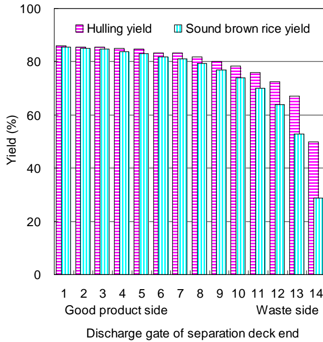
Figure 2. Hulling yields and sound brown rice yields of samples from 14 discharge gates of the separation deck end of a gravity separator.
