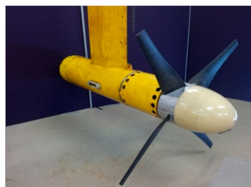
Figure 1. Tidal Turbine Testing (TTT) device and rotor.
