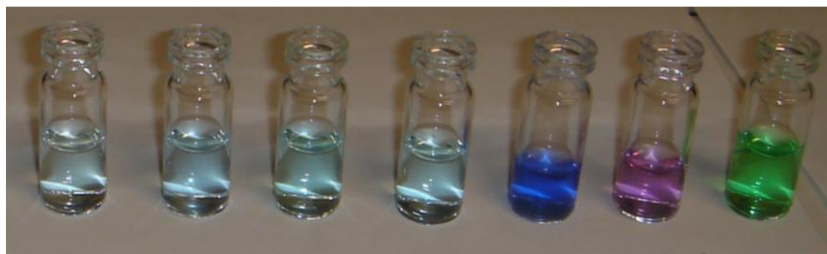
Figure 1.9 Colour change of receptor 53 in MeCN. From left to right: free receptor, +1Eq. F - , +1Eq. Cl - , +1Eq. Br - , +1Eq. CN - , +2Eq. CN - , +1Eq. I - . The image is reported according to Ref. 74.
