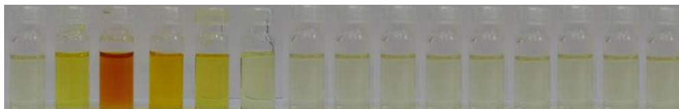
Figure 3.28 Colour change of L 21 (0.01M) in DMSO upon addition of 1 equivalent of the correspondent tetrabutylammonium anion salt (tetraethyl in the case of HCO 3 - ) (2.5 10 -2 M). From left to right: receptor, H 2 PO 4 - , F - , HPpi 3- , HCO 3 - , ADP, AMP, ATP, Mal - , Glu - , NO 3 - , CN - , ClO 4 - , Cl - , BzO - .
