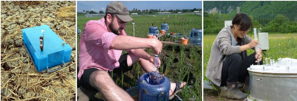
Figure 1. Examples of different non-steady-state chamber designs (Photo sources: Sebastian Weller, Baldur Janz, Gasche, 2017a).
