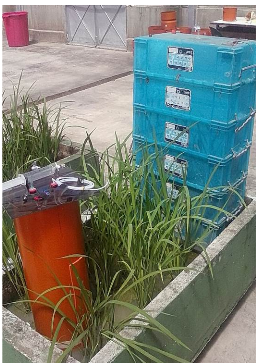
Figure 8. Example of chambers made of a waste-water pipe and stackable plastic containers.
