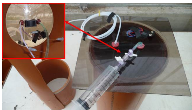
Figure 1. Modified waste-water pipe with base frame and detail of the inside of the pipe/chamber.
