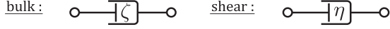
FIG. 6. The bulk part (left) and the shear part (right) for a Navier-Stokes (or Newtonian) fluid. A dashpot yields a viscous stress proportional to the time derivative of the induced metric.
