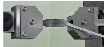
(b) Specimen fixed to the tensile machine
