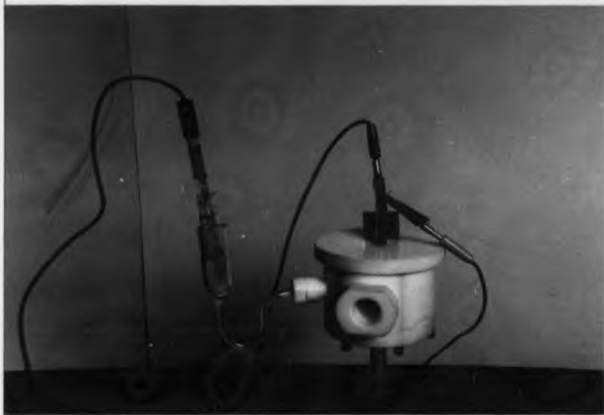
Fig. 3. 4. The electrochemical cell used for the photoelectrochemical experiments.
