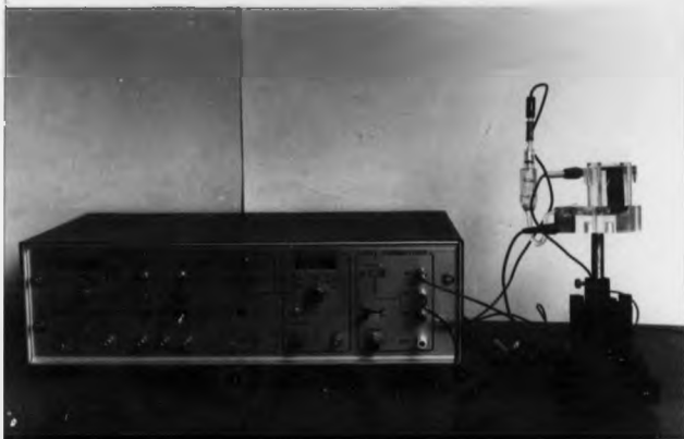
Fig. 3. 7. A cell used in the in-situ EXAFS experiments to study films passivated both electrochemically and by immersion into the solution.
