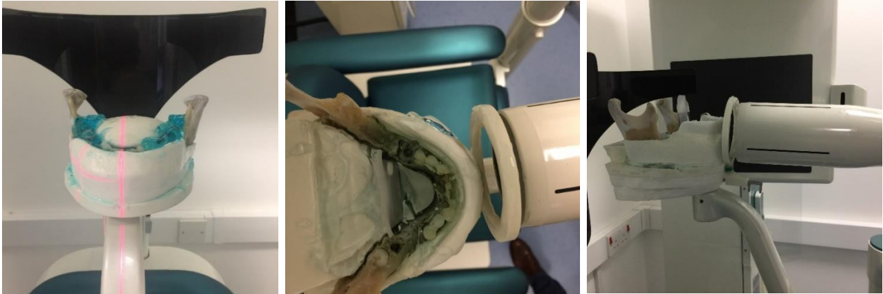
Figure 4-8. Set up demonstrating positioning of the phantom within the Morita Accuitomo 170 scanner and additional set up for periapical radiography. Note the slots posterior to the mandible in which size 2 plates could be placed at 0° or 15° from the perpendicular axis to the incisal edge.
