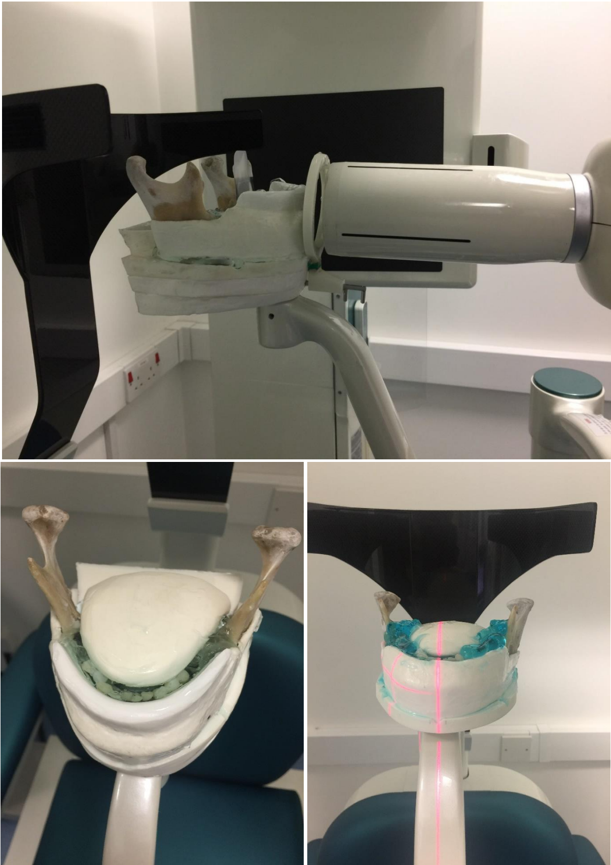
Figure 4-6. Top: phantom set up for PA radiography still within CBCT machine. Removal of the tongue analogue allows placement of phosphor plate and beam aiming device. Below: phantom in CBCT set up for scanning with tongue analogue in situ. Note the ultrasound jelly placed between soft tissue analogues to replicate saliva and to eliminate air pockets.
