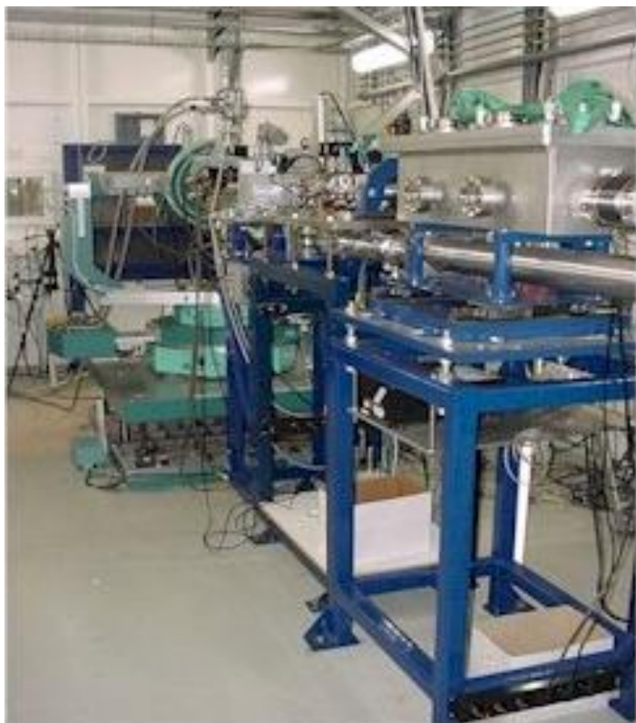
Figure 5.9 : Looking toward the diffractometer in the experimental hutch for XMas beamline 28 in the ESRF, taken from (A)
