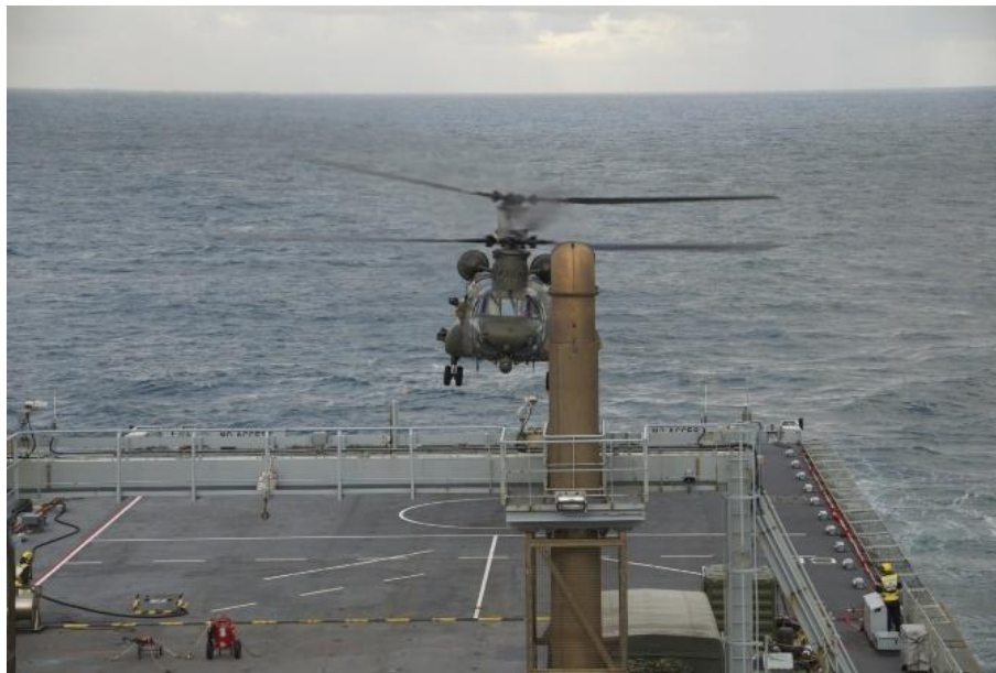
Figure 5.2 Ship exhaust discharging over helicopter deck. Photo by Courtesy of Lt Cdr RN L S Evans
