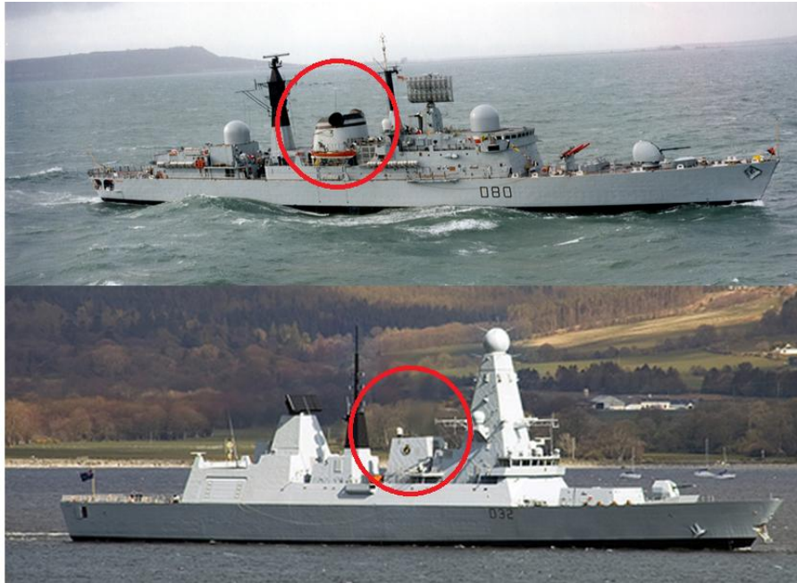
Figure 5.1 Funnel designs of the Type 42 (top) and the Type 45 (bottom)
