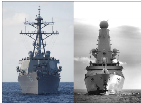
Figure 1: Mast profiles of a US Arleigh-Burke class and a UK Daring class destroyer
