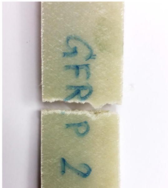
Figure 4.5: Failure modes in the GFRP woven composite laminates under in-plane shear loading.
