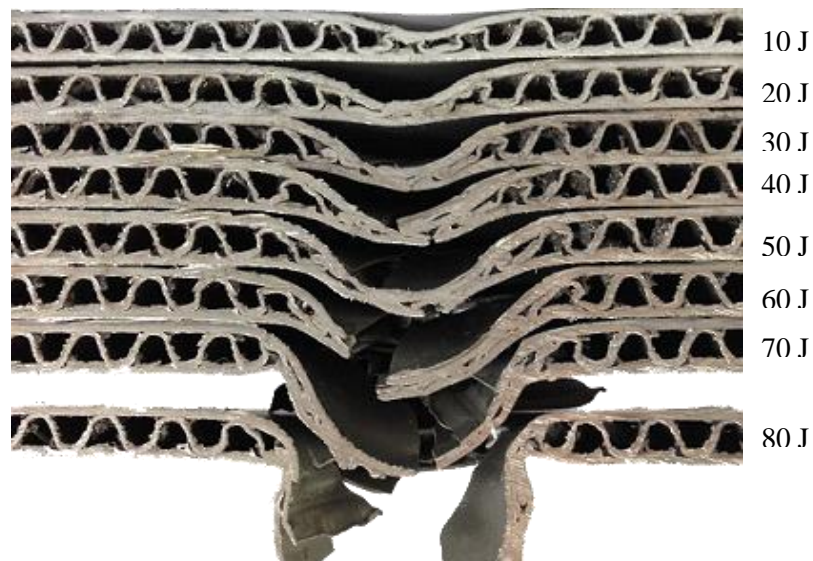
Figure 5.5: The process of damage development in the 6 mm thick panel.
