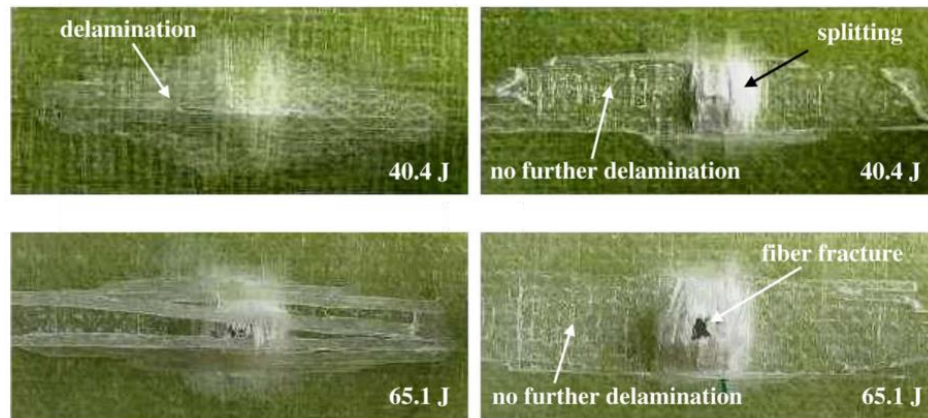
Figure 2.35: Bottom layer delamination and fiber failures [87]
