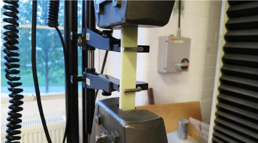
Figure 3.23: Instron 4204 universal testing machine and mechanical extensometer.
