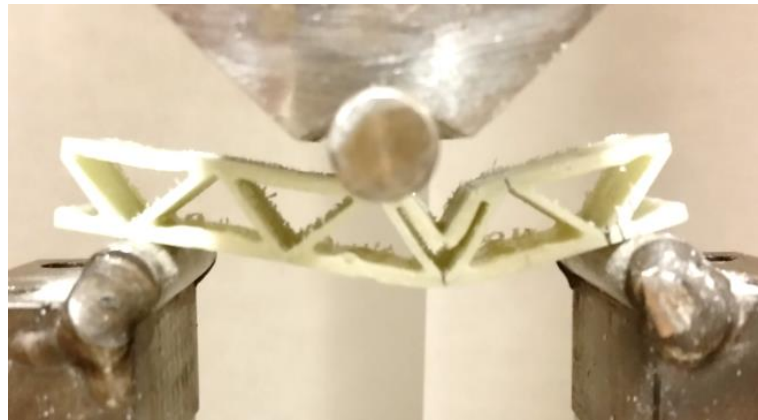
Figure 4.15: The plain GFRP corrugated-core undergone by three-point bending test.
