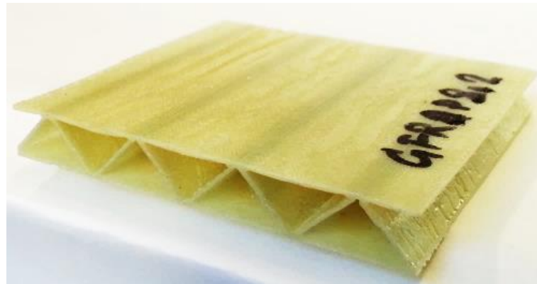
Figure 3.12: Photograph of a plain GFRP triangular corrugated sandwich structure without an embedded foam.
