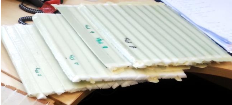
Figure 3.8: The sample panels after cured from hot press process.
