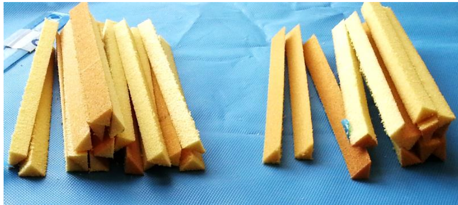
Figure 3.4: Foam core elements cut into a prism shape.
