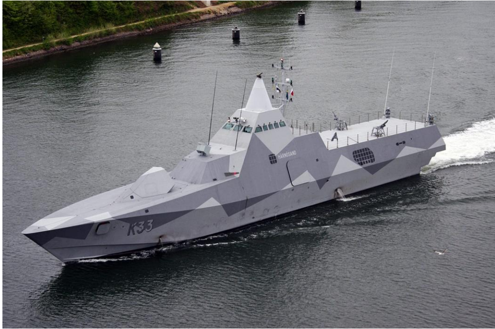
Figure 1.5: The image of the newest Visby class corvette that the whole superstructure was built by using composite material[8].
