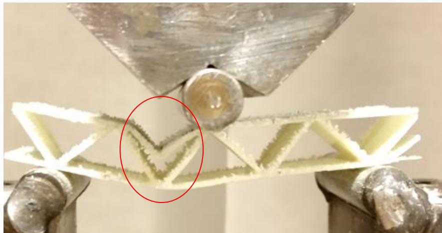
Figure 4.8: GFRP triangular corrugated-core under three-point bending test.
