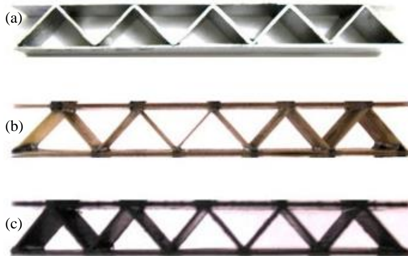
Figure 2.17: Triangular corrugated-core sandwich structures made of (a) Aluminium 2024 O (b) GFRP (c) CFRP [28].
