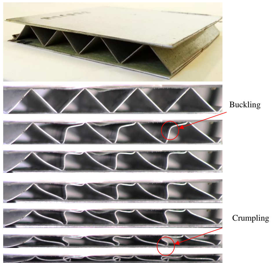
Figure 4.50: The process of damage development of the hybrid sandwich panel based on triangular corrugated and 1/1 FML core.
