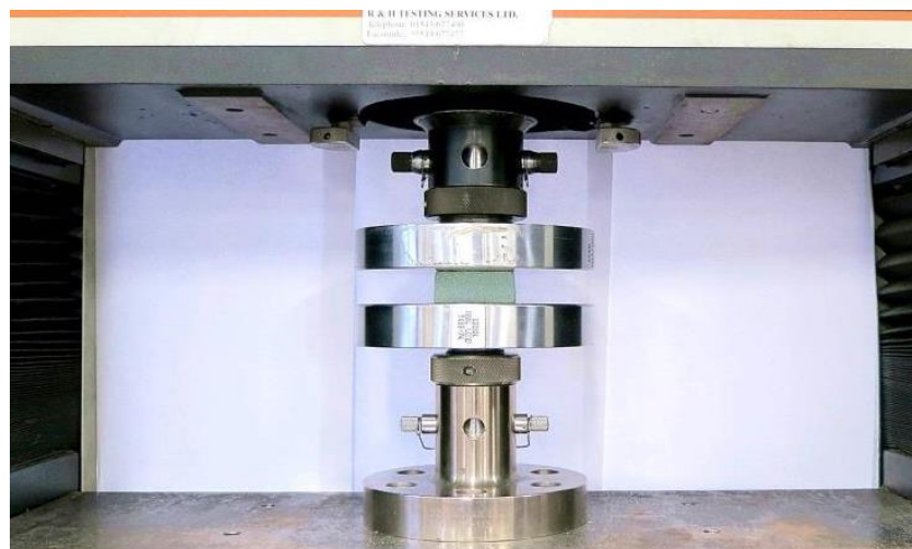
Figure 3.26: The square foam specimen under compression testing.
