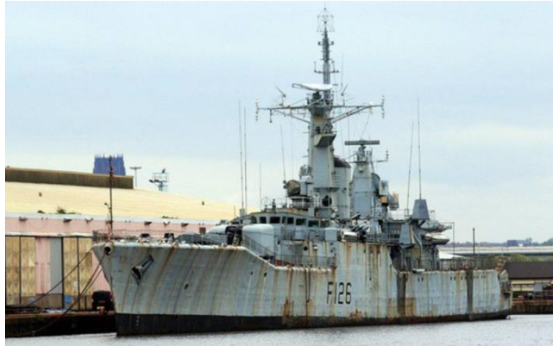
Figure 1.4: Illustrates the battle ship experiences with a severe corrosion around the superstructures[7].
