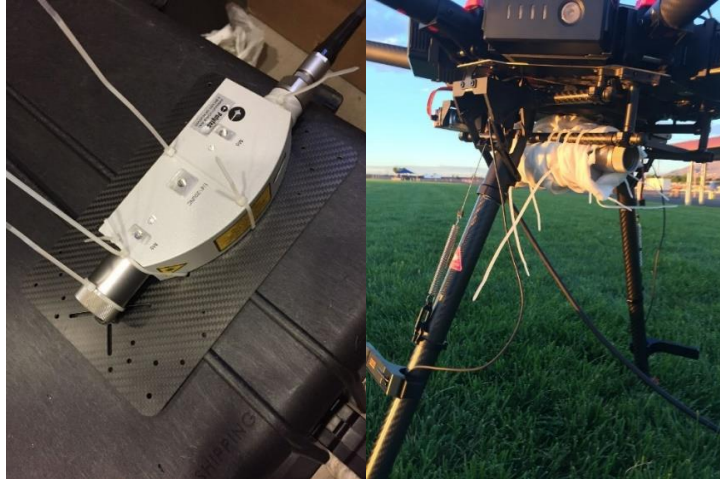
Figure 4-17. Vibrometer assembly to the UAS.
