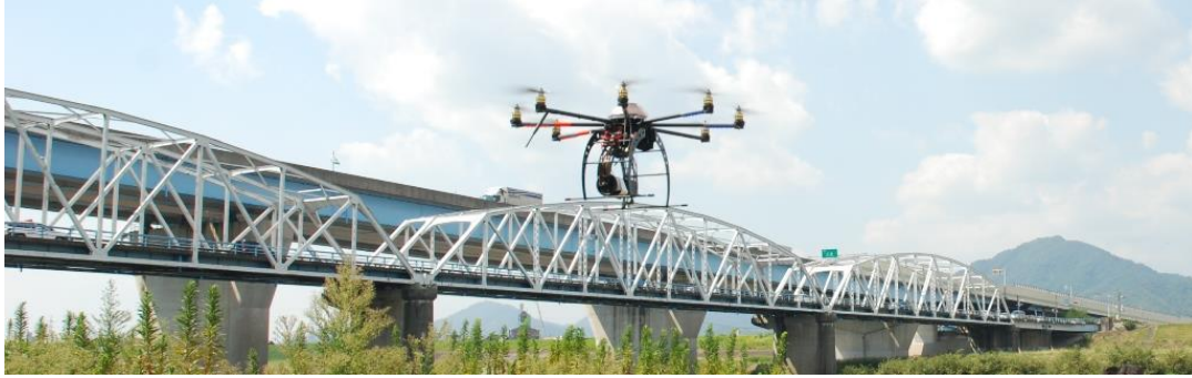
Figure 2-9. UAS for bridge monitoring (Smart Sensys 2017)
