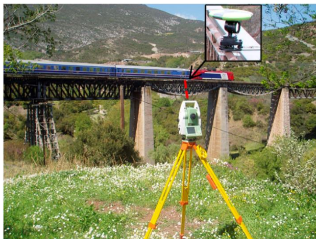
Figure 2-5. Railway bridge monitoring using a robotic total station (Psimoulis and Stiros, 2013)
