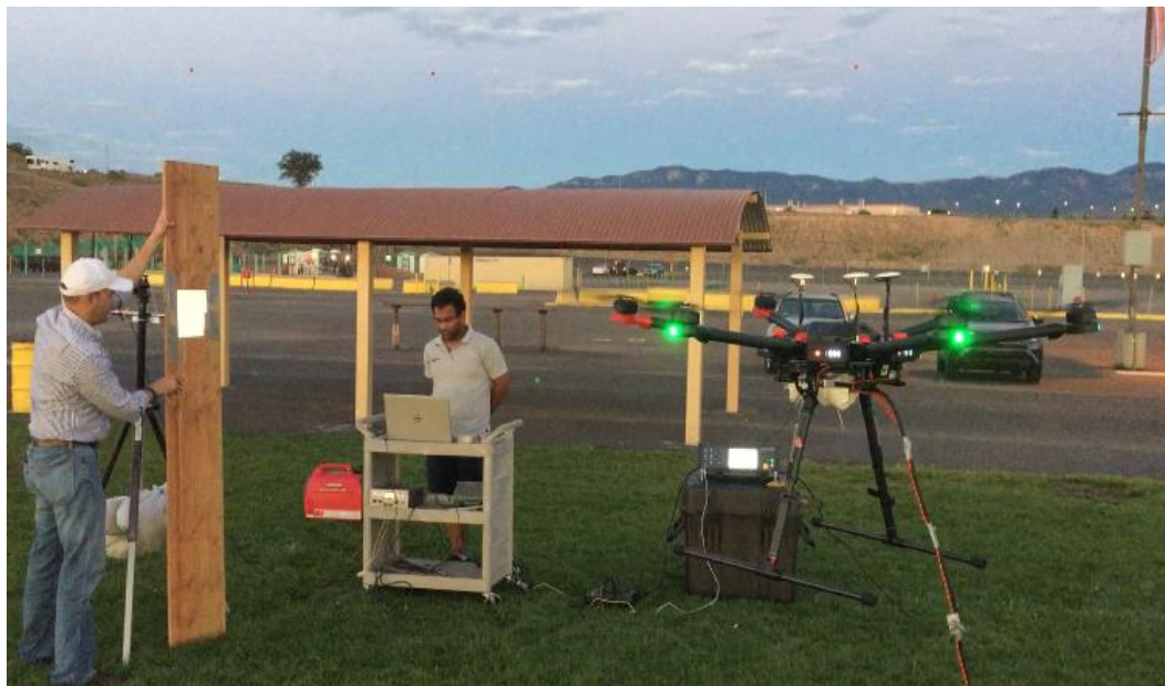
Figure 4-16. Filed testing using a LDV mounted on a UAS
