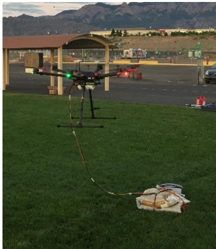
Figure 4-18. UAS tethered to the ground along with vibrometer cable.
