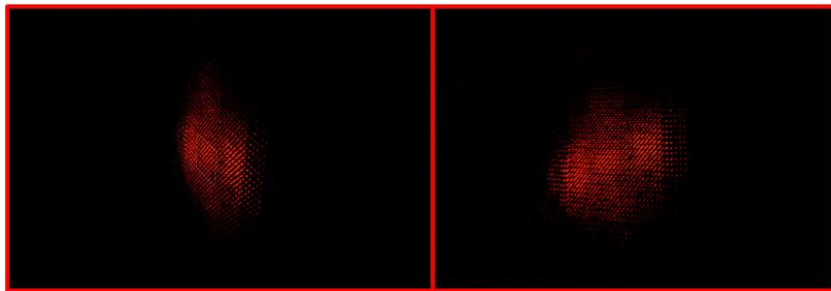
Figure 3.31 Top: Camera perspective to the neon bulb array. Left: image of unrectified neon bulb array. Right: rectified image of neon bulb array.
