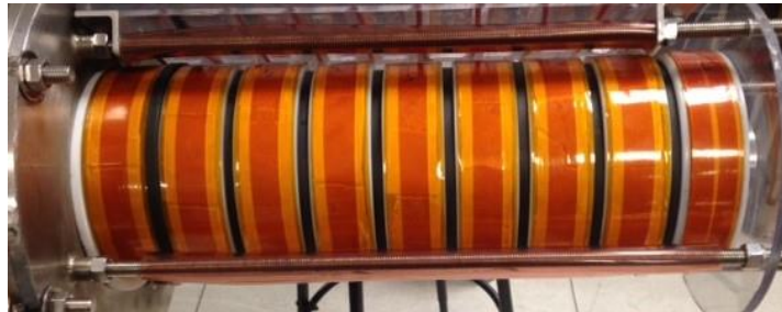
Figure 3.9 Solenoid electromagnet used on the SINUS-6 accelerator which is composed of 9-coils. The Solenoid is approximately 40 cm long, can produce a magnetic field of 2 Tesla (T), and is composed of 488 turns of 16 AWG copper wire.
