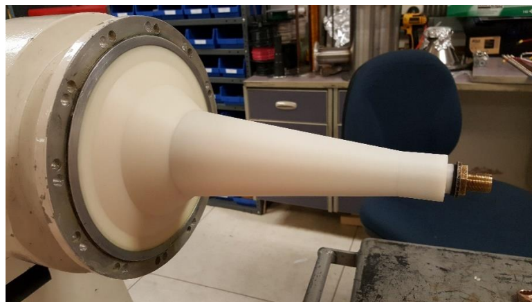
Figure 3.7 Magnetically insulated oil-vacuum interface.
